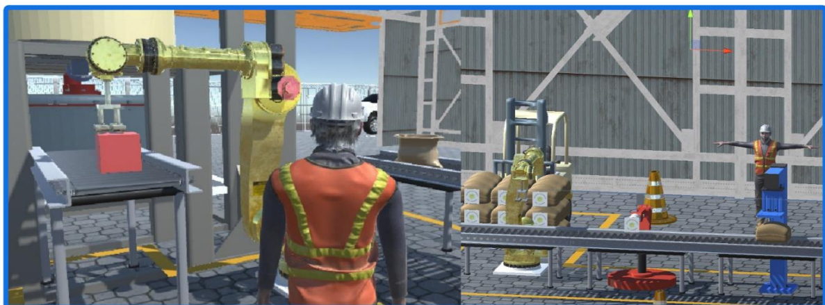
Figura 11. Virtualization of the automatic gelatin weighing and packanging process.
