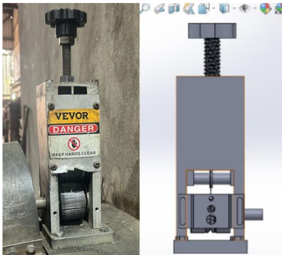
Figure 2. Example of manual wire stripping machine head and designed model
